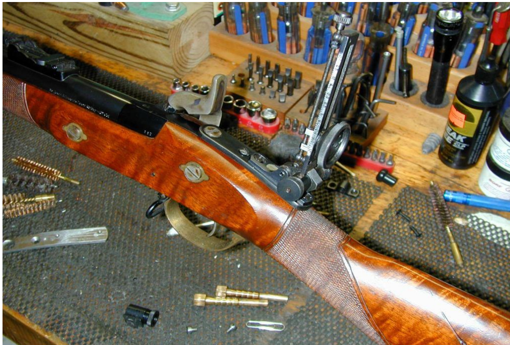
Picture shows a reproduction sight base extension to fit a Creedmoor sight to a British target rifle without drilling holes into the wood.
